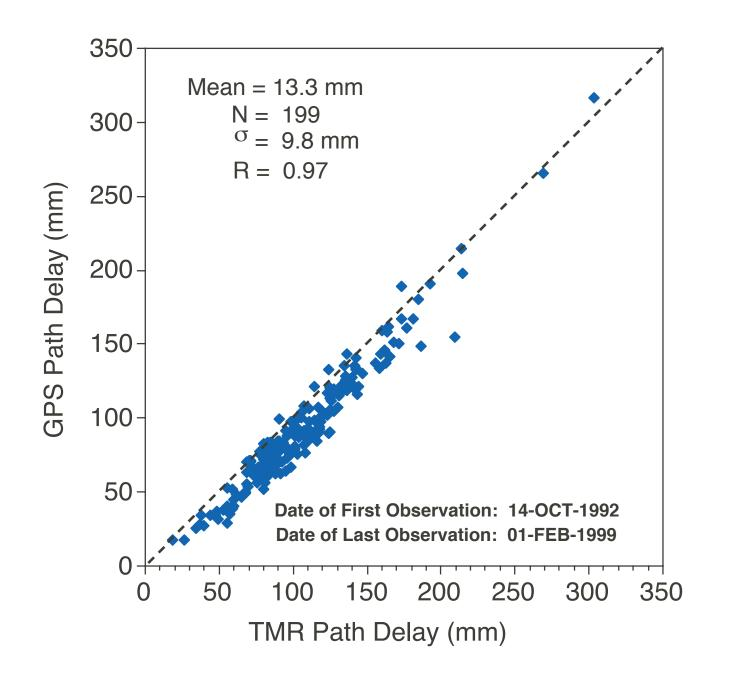
The close agreement between the TMR- and GPS-based PD estimates hints at the possibility of using time series of the differences for detecting subtle drifts in the radiometer. Provided in the following schematic are drift estimates (TMR–GPS) for the 11 station/pass pairs considered in the study:
