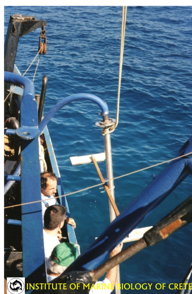
The present situation at Gavdos pier and instrument location installations. Deployment of the Wave & Tide Record was in May 2002 at a depth of 10 m.
