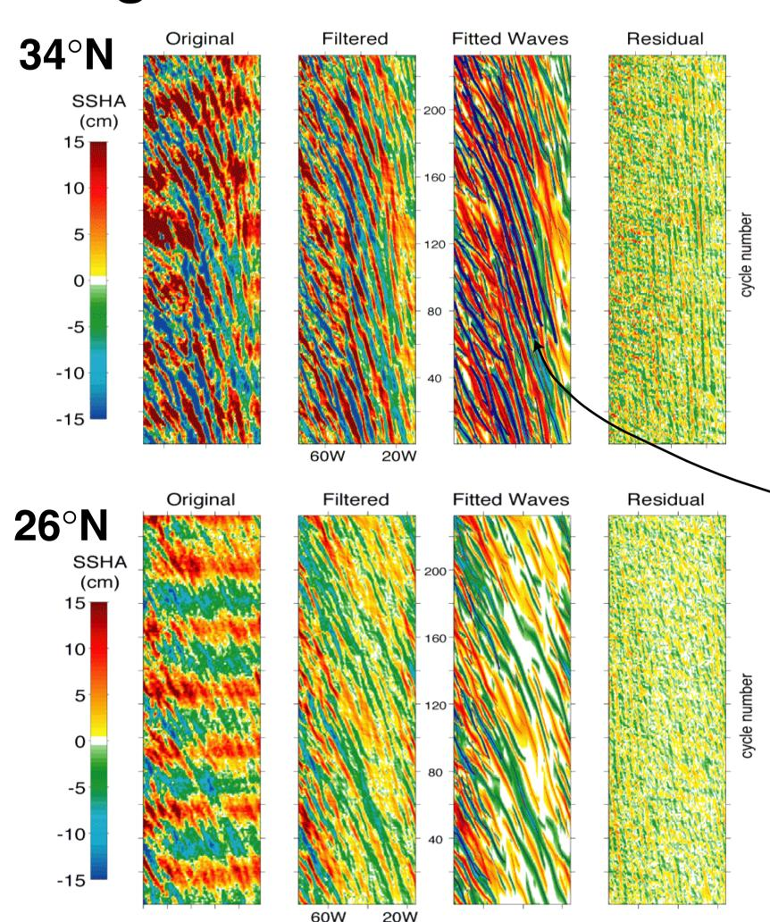
The third subplot shows the tracks of the fitted downwelling (red) and upwelling (blue) waves. For each of those we now have the values of the parameters in each point of the track
