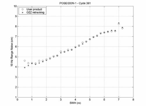
a very good consistency between the POSEIDON-1 ground retracking and the OZZ retracking
