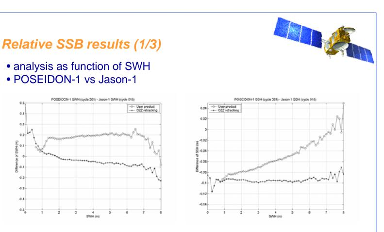
• The fact that after OZZ retracking the difference of SSH is a constant and does not show any SWH dependency indicates that the SSB of the two altimeters is very similar
