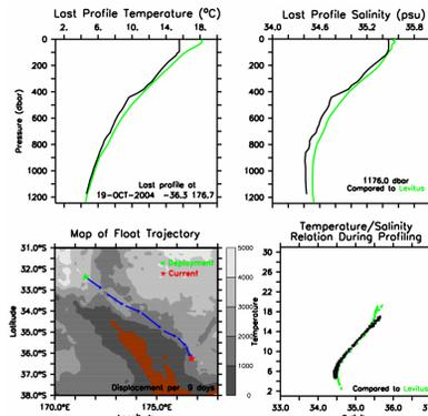
2 Argo floats provide T and S profiles and 1000 m reference velocity every 10 days. This float is following the East Auckland Current.
