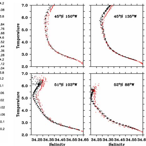
7 T/S diagrams from Argo float profiles located near WOCE lines show consistent fresh offsets at temperatures warmer than 5°C. All floats used here were new enough so that drift in salinity calibration was not significant.
