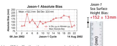
The bias (SSH offset) estimates were calculated for the calibration phase (Jason-1 cycles 1-22). The Jason-1 bias appears to be more variable than the T/P bias. Using only common cycles, the relative bias is  $+150 \pm 11$  mm. Uncertainties have been calculated from a formal error budget.
