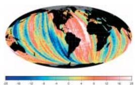
Geographically correlated orbit errors (Jason-1 GDR orbit – JPL GPS orbit). Only descending passes shown. Figure from Haines et al., 2004, included with permission.
