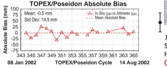
above t Height a True SSH TOPEX/Poseidon Sea Surface Height Bias:  $0 \pm 14 \text{ mm}$
