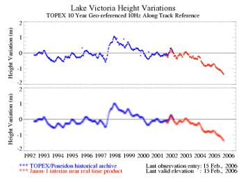
Time series of lake and reservoir elevation variations using archived Topex/Poseidon and near-real time Jason-1 data products.
