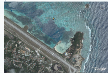
GLOSS/CLIVAR tide gauge Point La Rue collocated with a DORIS station in Mahe Island (Seychelles)
