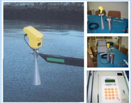
Figure 3. Radar tide gauge devices ready to be installed at l'Estartit harbour. This modern installation will work in a parallel way to the classical floating gauge active since 1992. Details of the electronics are shown in the images above and a final deployment is presented in the image below (example of the installation at Vilagarcía de Arosa Port, Spain). Images and deployments provided by Geonica sl, Earth Sciences.
