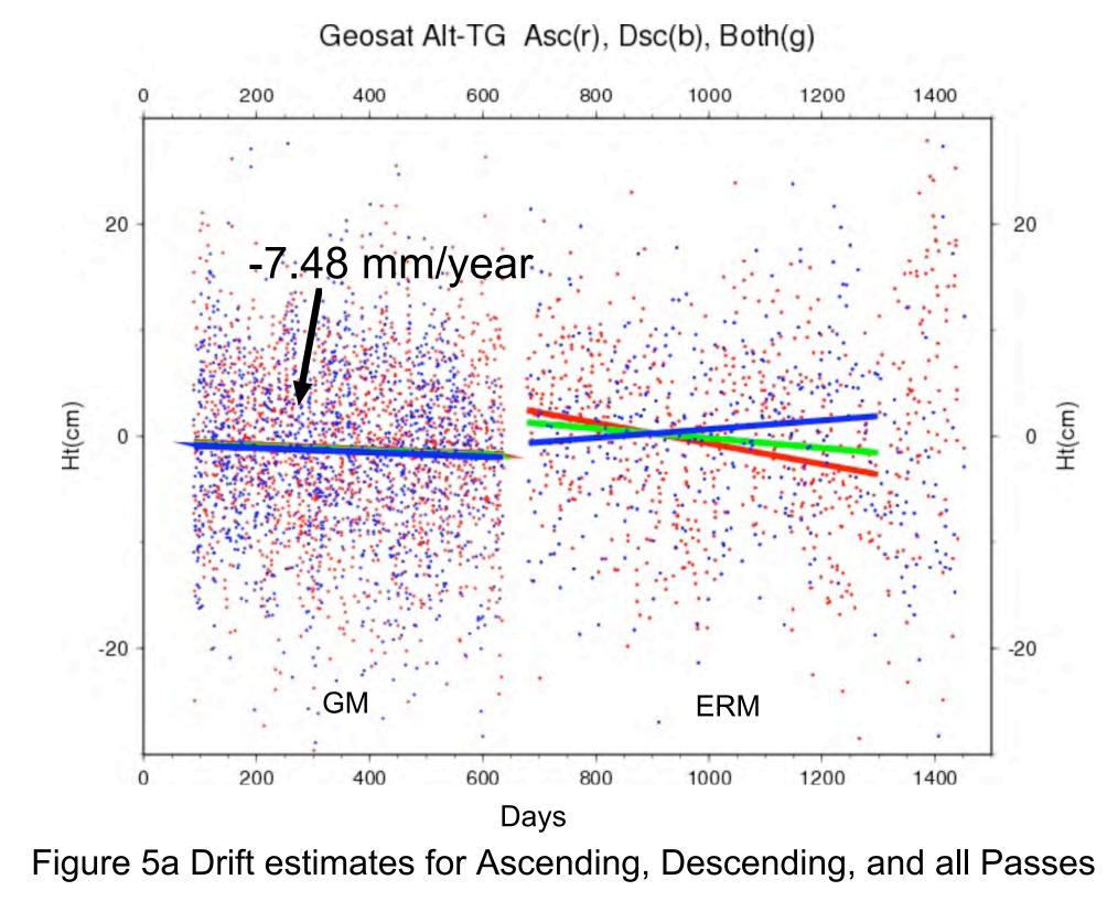
Figure 5a (left) shows the drift estimates (Geosat -Tide Gauge) computed separately for ascending, descending, and all passes . For the GM, the three curves fall almost exactly on top of each other, with an average of -7.48 mm/yr. The ERM shows diverging estimates, perhaps due to having fewer samples, poorer orbits and greater ionosphere errors.
