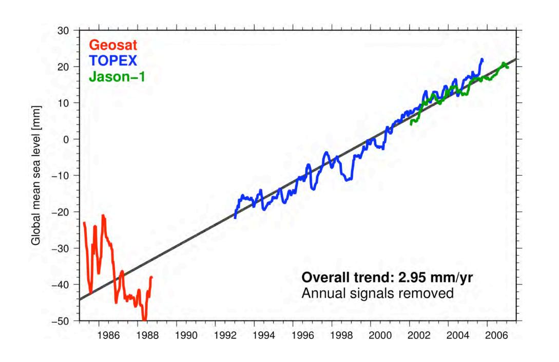
Figure 1. Global mean sea level change from Geosat, TOPEX and Jason-1, based on a simultaneous fit to a single trend and annual function and separate bias estimates for each satellite.
