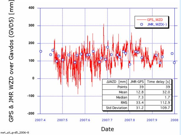
Comparison of GPSderived WZD at GVD5 (30 min averages) with JMR values obtained from GDR-C release.
