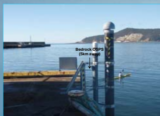
Fig.2 The Burnie tidal gauge and co-located CGPS. A second "bedrock" CGPS is located at Round Hill approximately 5km away.
