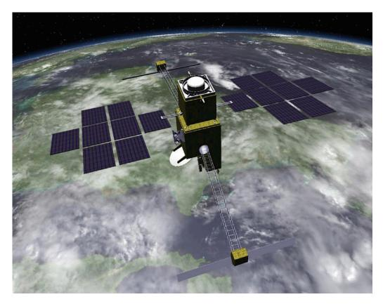
The SWOT spacecraft, shown here in an artist's conception, will make accurate measurements of mesoscale ocean features and surface water parameters.
