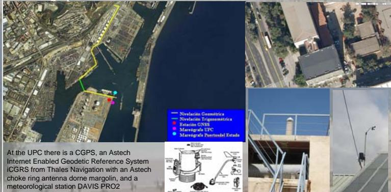
At the UPC there is a CGPS, an Ashtech Internet Enabled Geodetic Reference System (ICGRS) from Thales Navigation with an Ashtech choke ring antenna dome margolin, and a meteorological station DAVIS PRO2
