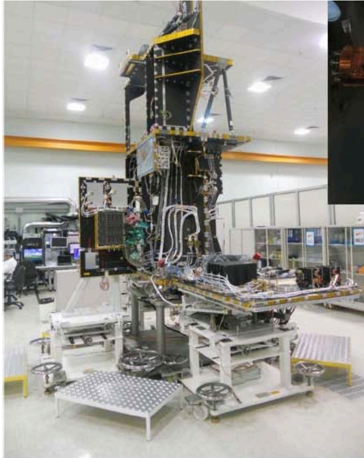
Platform Module undergoing electrical Integration Test (courtesy of TAS-I)
