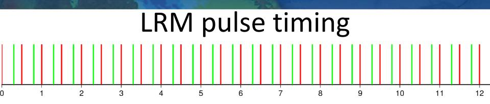
In a conventional LRM instrument, transmit and receive are *interleaved* and go on alternately, each at approximately 2 per millisecond (PRF ~= 2 kHz).
