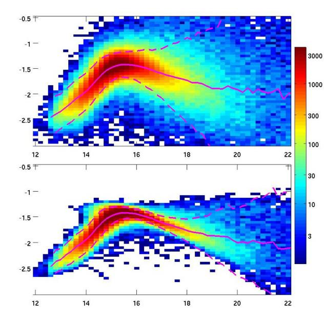
Sigma0\_Ku – Sigma0\_C a a function of Sigma0\_C Top uses data from MLE-4; bottom after adjustment A reminder that offset in bias between 2 different retrackers (e.g. when switching from open ocean to coastal) will in general be a function of wave height and sigma0 i.e. equivalent to requiring a slightly different SSB model for each retracker
