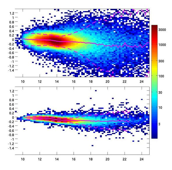
Sigma0\_Ku difference (Jason2-Jason1) as a function of Sigma0\_Ku Top uses data from MLE-4; bottom after adjustment 3) The empirical relationship between Kuand C-band values becomes much tighter, meaning that a reliable rain flag can be applied to edit SSH data that are affected by rain.
