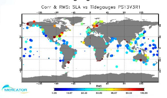
RMS misfit in mm between SLA and tide gauges in 2010, the dot size increases with the correlation (large=corr>0,75).
