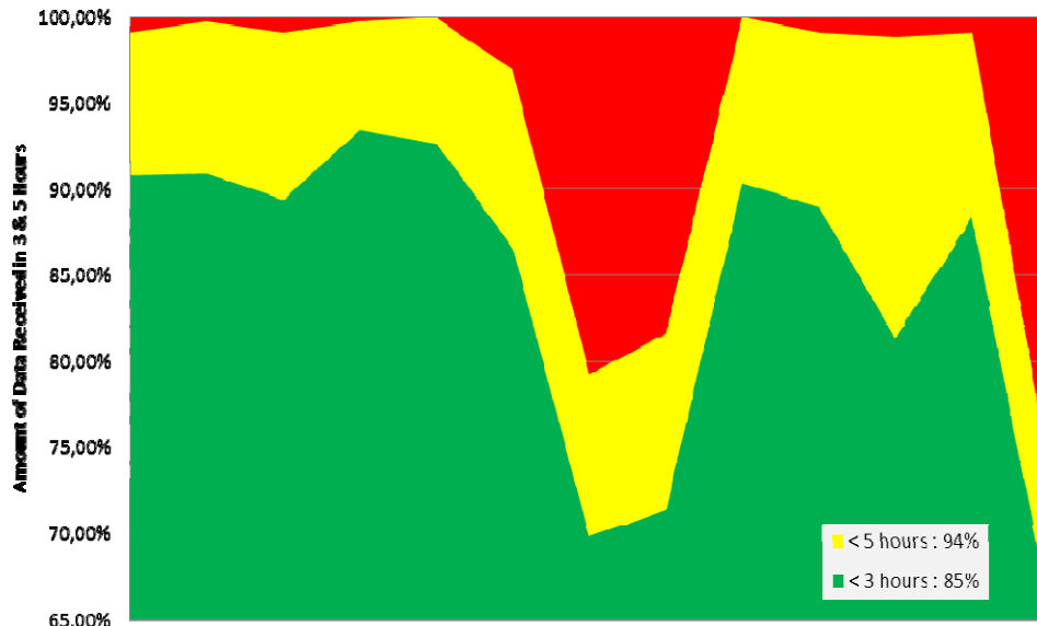
Jason-2: Sep-2012 through Sep-2013 Monthly OGDR Latency Statistics (measured at end users EUMETCast Reception Station)
