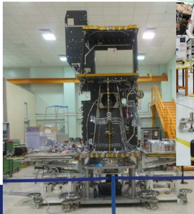
S3B Platform undergoing electrical integration at Platform Responsible facilities in Rome (I)
