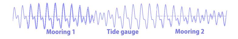
Determine mooring to TG offsets using a harmonic analysis of time series differences (dominated by M2, Amp = 0.126 m). RMS of the non-tidal residual, (mooring – tide gauge) is 22 mm (reduces to 20 mm when differential effect of air pressure is considered).
