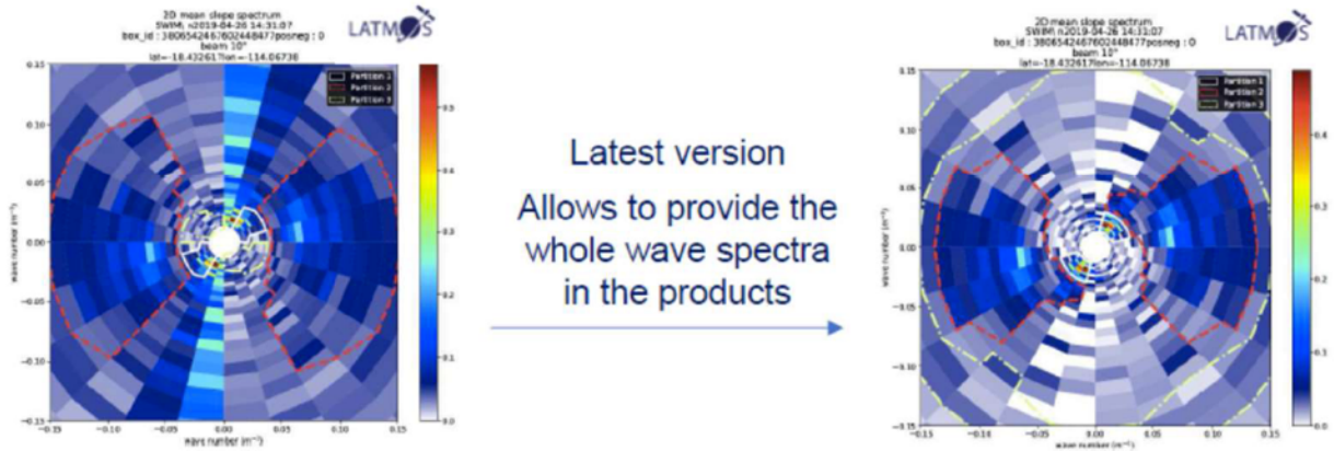
Figure 3.2-3. The strong change in derived 2D ocean wave spectra in the along-track direction with the latest version product clearly being improved
