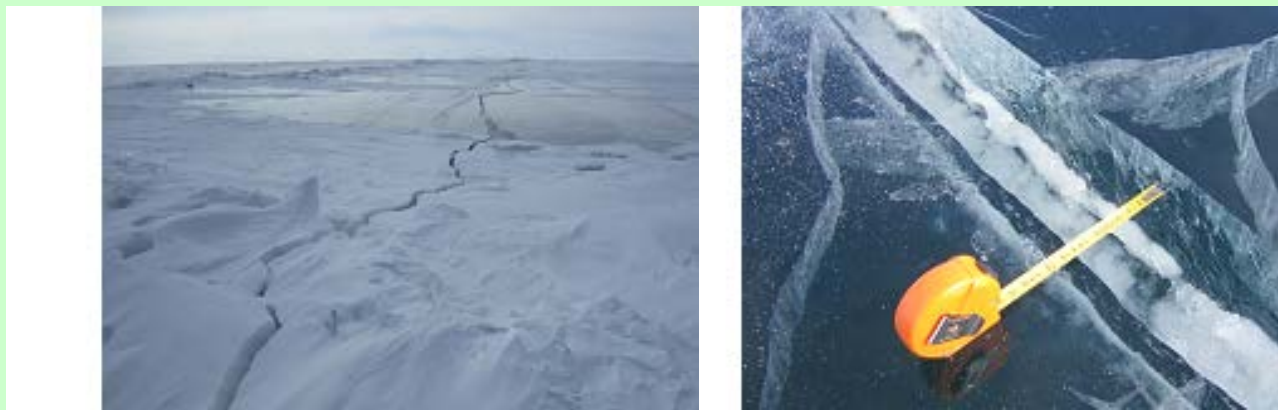
A secondary ice fracture (formed 10 min ago) Width - 6 cm, ice thickness 110 cm, level difference - 2 cm
