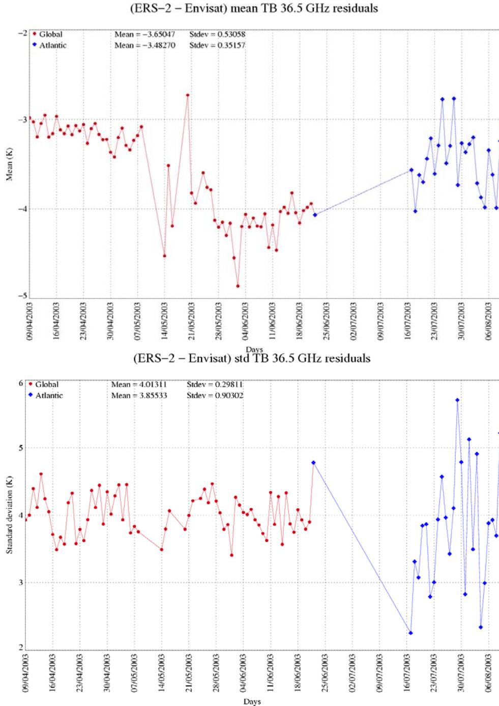
**Figure 101 : Mean and standard deviation of (ERS-2 – Envisat) TB 36 GHz along track residuals for each day.**
