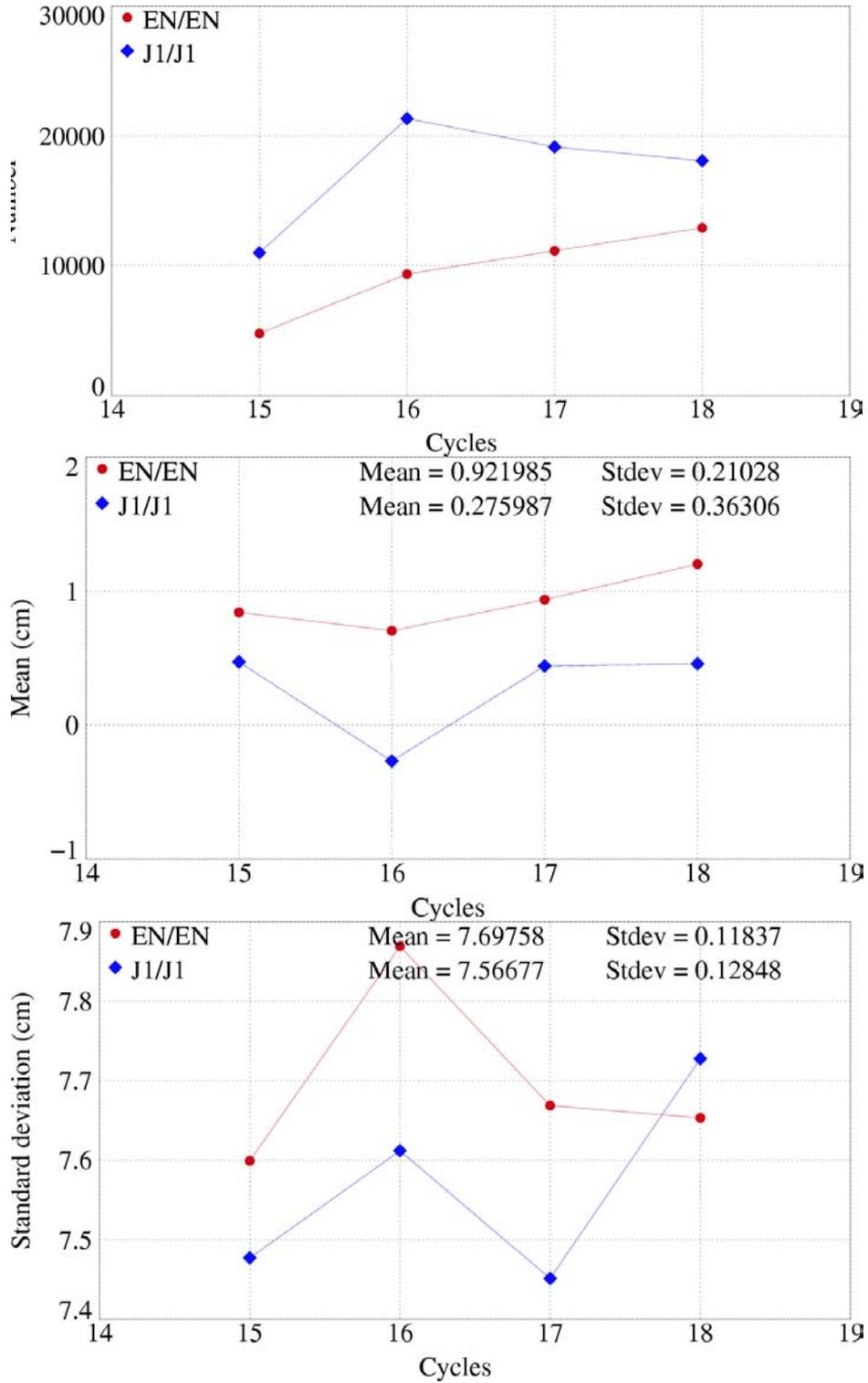
**Figure 91 : Number, mean and standard deviation of SSH differences at crossover (cm),  $|\text{latitude}| < 66^\circ$ , Bathy < -1000m**
