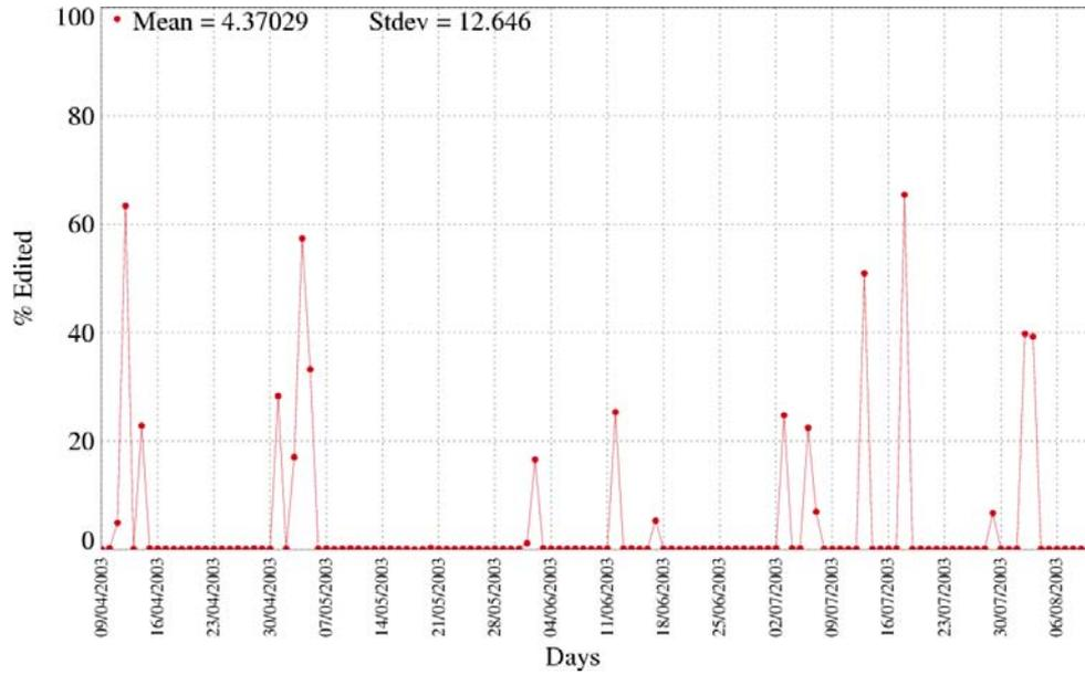
**Figure 6 : % of measurements edited because of the S-Band anomaly over ocean**
