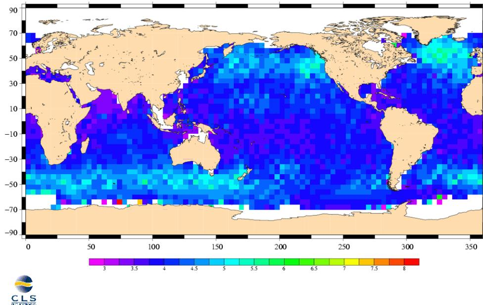
**Figure 61 : Standard deviation of Jason-1 High Frequency signal, using 20Hz data**
