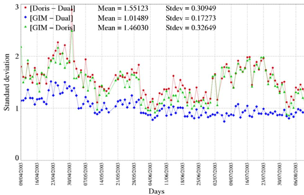
**Figure 22 : Standard deviation of [Doris-Dual], [GIM – Dual] and [GIM-Doris] ionospheric correction (cm)**
