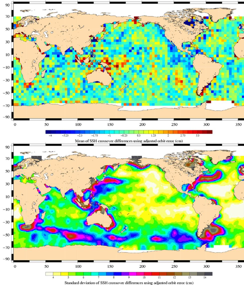
**Figure 90 : Geographical pattern (4x4 degree bins) of crossover [Envisat – Jason-1] mean and standard deviation SSH differences using adjusted long wave length error (cm), from cycle 15 to cycle 18**
