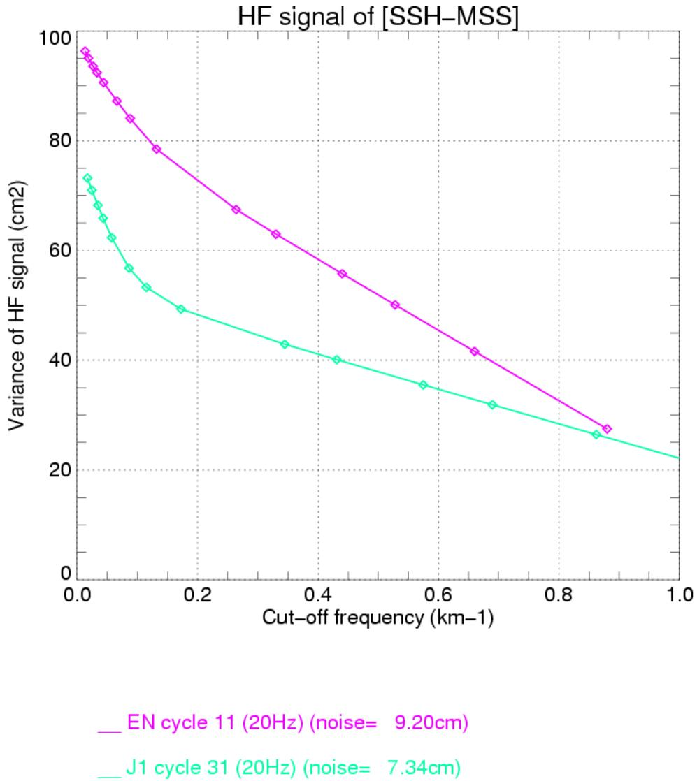
**Figure 59 : Standard deviation of HF[SLA<sub>nc/mss</sub>] at 20Hz according to the cut-off frequency**
