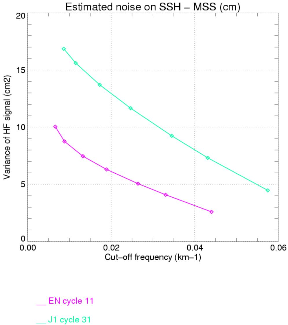
**Figure 68 : Standard deviation of High Frequency signal as a function of the cut-off frequency, using 1Hz data**
