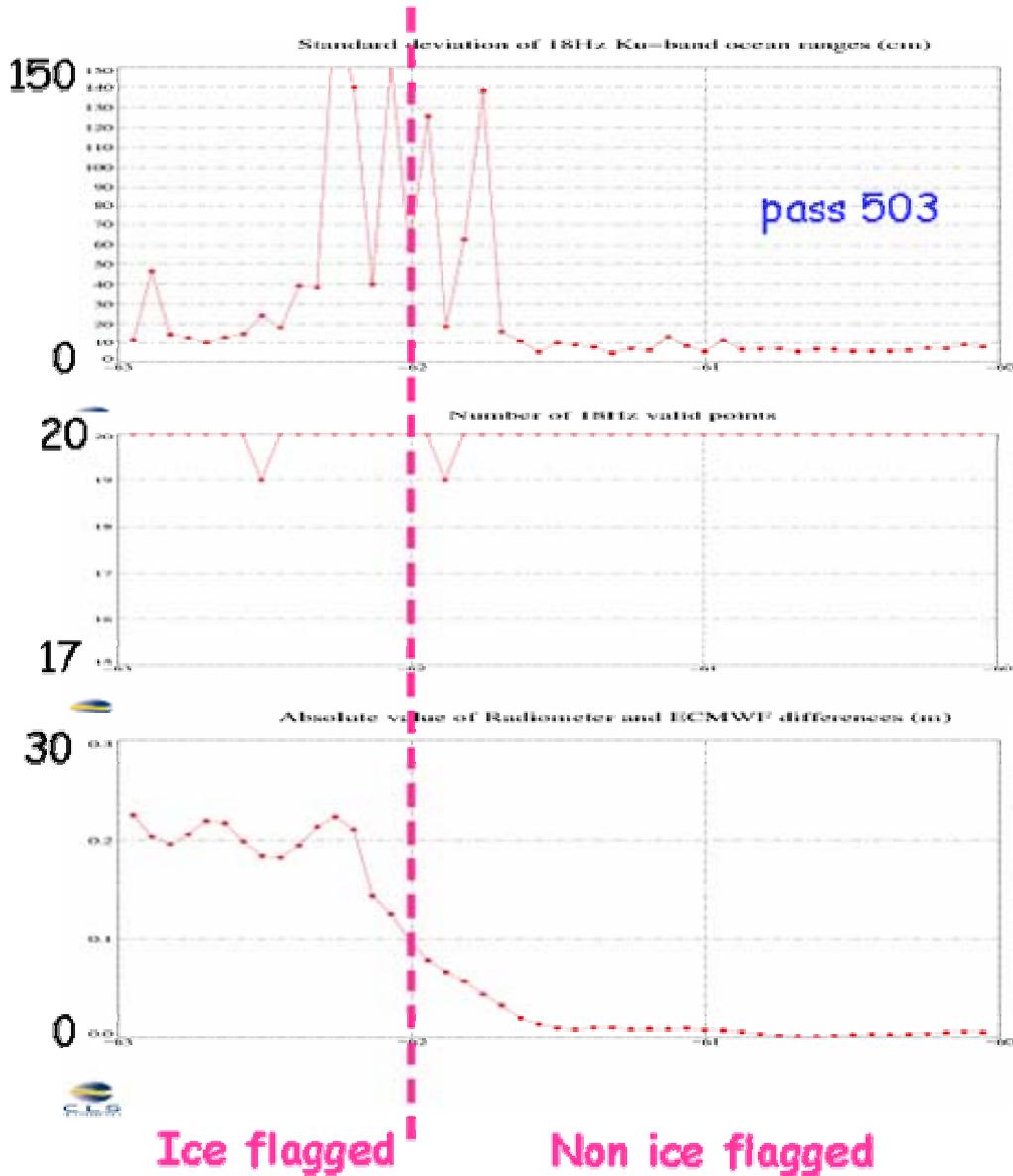
Figure 48 : RMS of Ku-band range, number of elementary measurements, and |MWR-ECMWF| on pass 503
