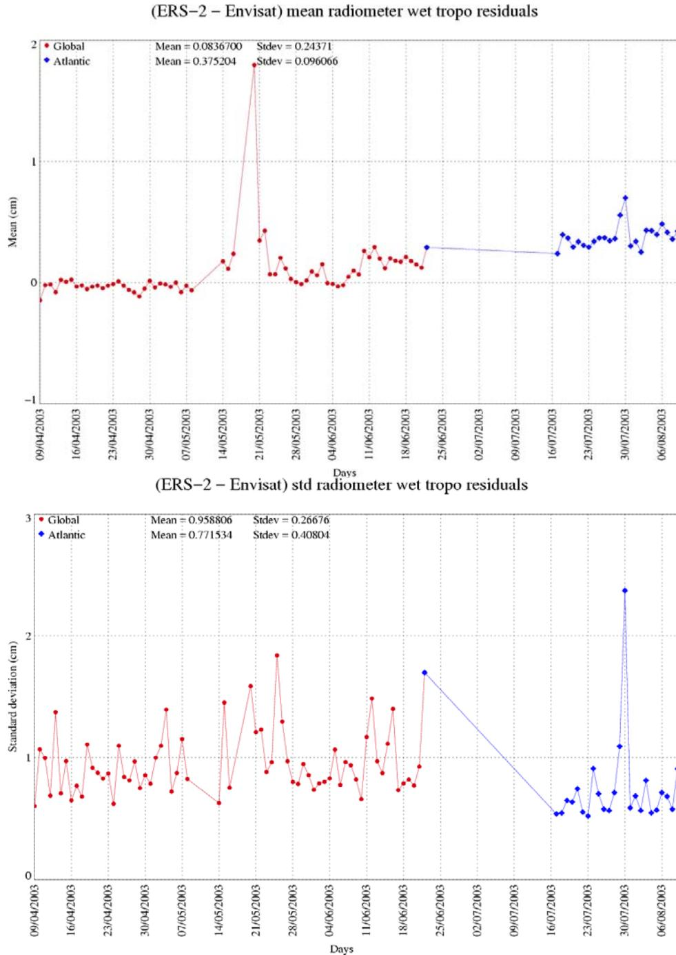
**Figure 99 :** Mean and standard deviation of (ERS-2 – Envisat) Radiometer wet troposphere correction along track residuals for each day.
