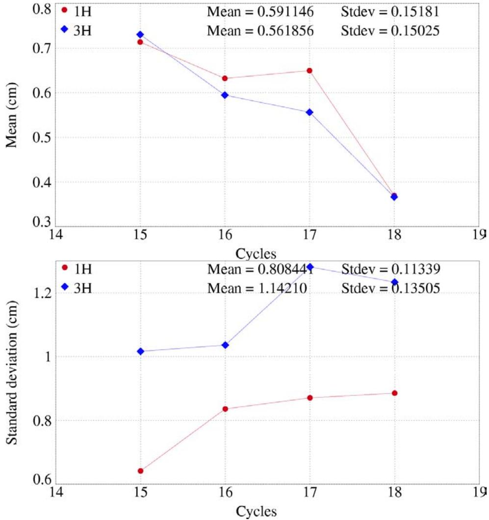
**Figure 85 : Mean and standard deviation of [Envisat – Jason-1] Radiometer wet troposphere correction differences at crossover (cm)**
