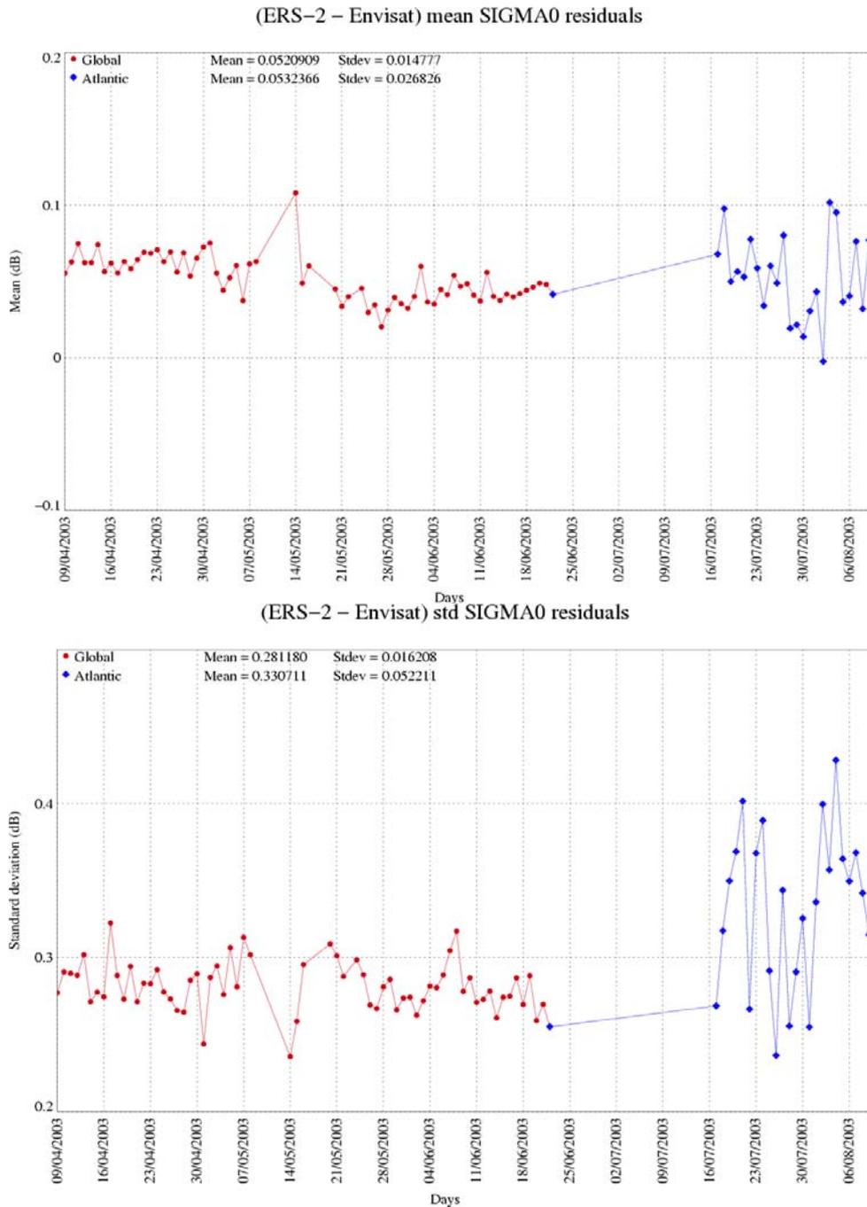
**Figure 98 :** Mean and standard deviation of (ERS-2 – Envisat) SIGMA-0 along track residuals for each day.
