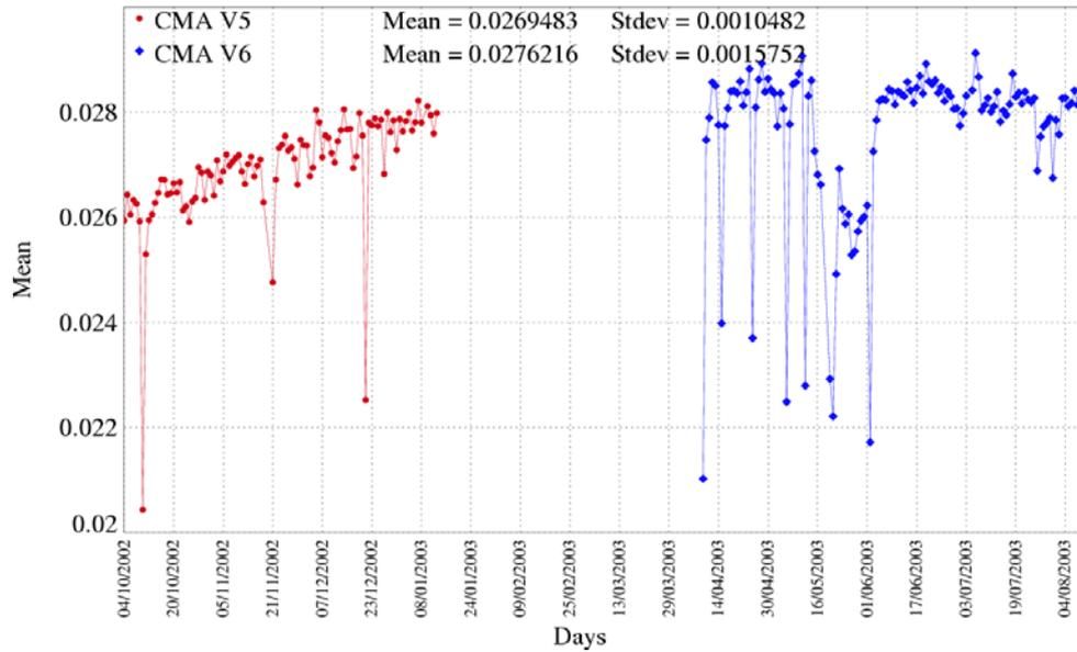
Figure 19 : Mean of off-nadir angle from waveforms (deg2)
