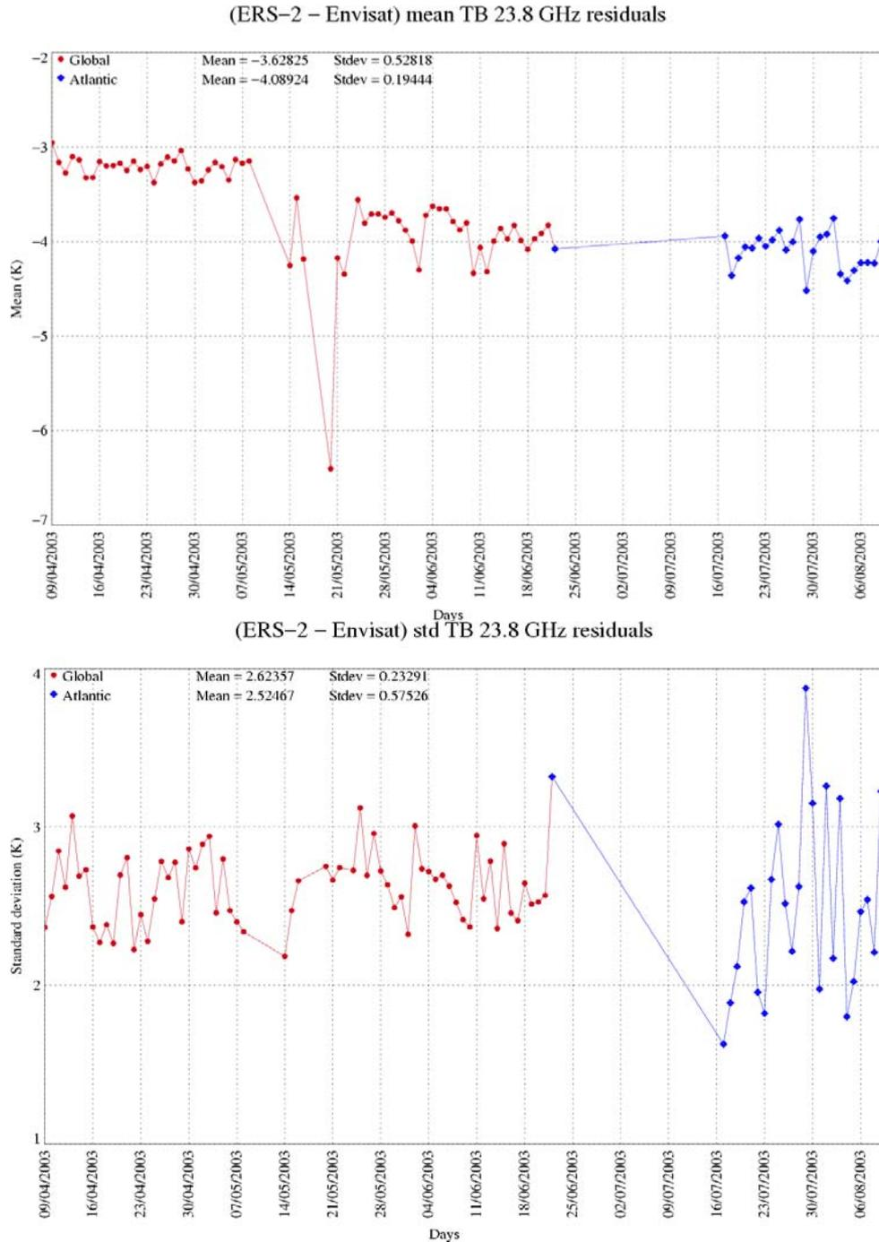
**Figure 100 : Mean and standard deviation of (ERS-2 – Envisat) TB 23 GHz along track residuals for each day.**
