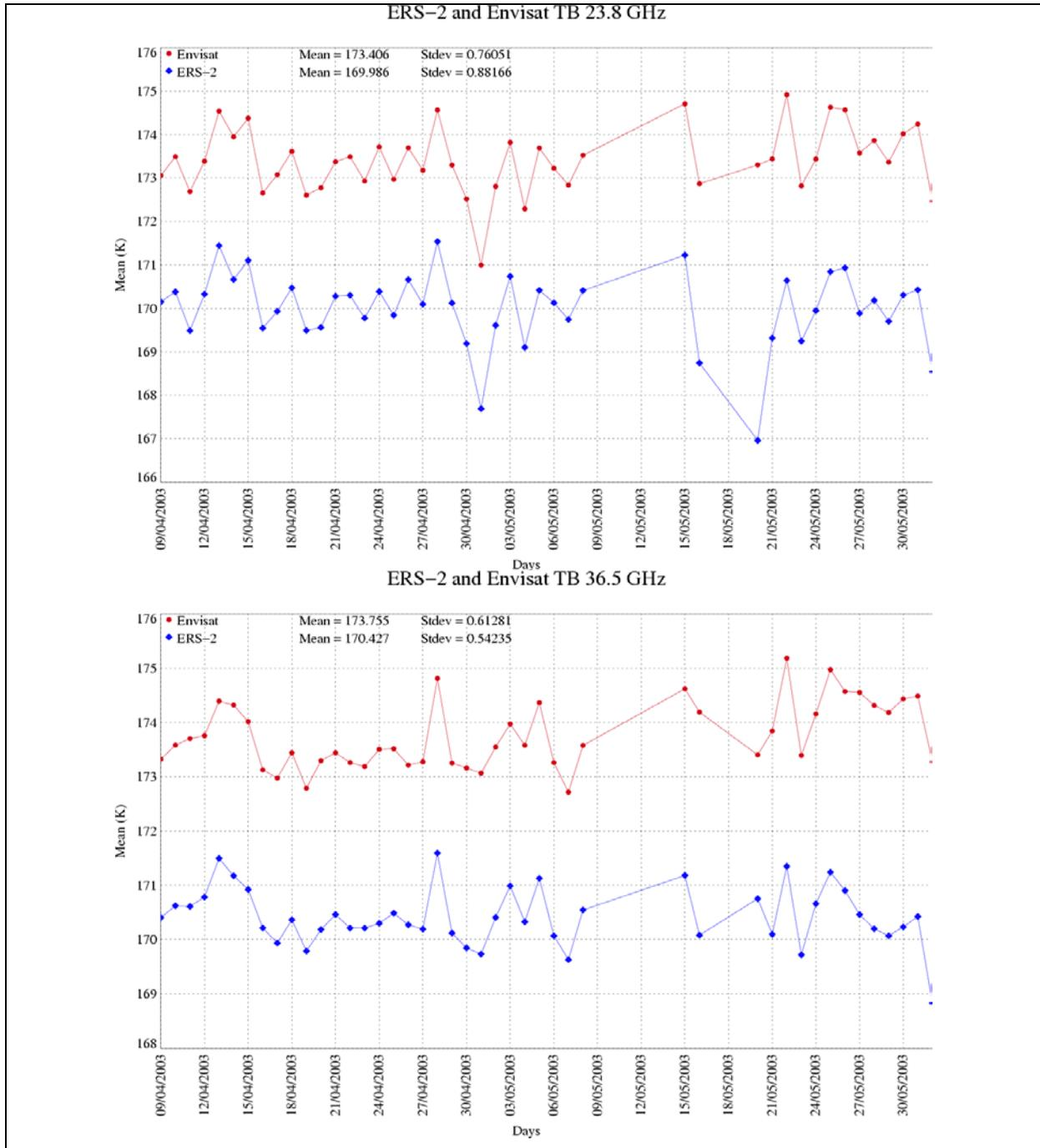
**Figure 102 : Mean of ERS-2 and Envisat TB 23.8 GHz (top) and 36.5 GHz (bottom) for each day of cycles 15 and 16 Envisat**
