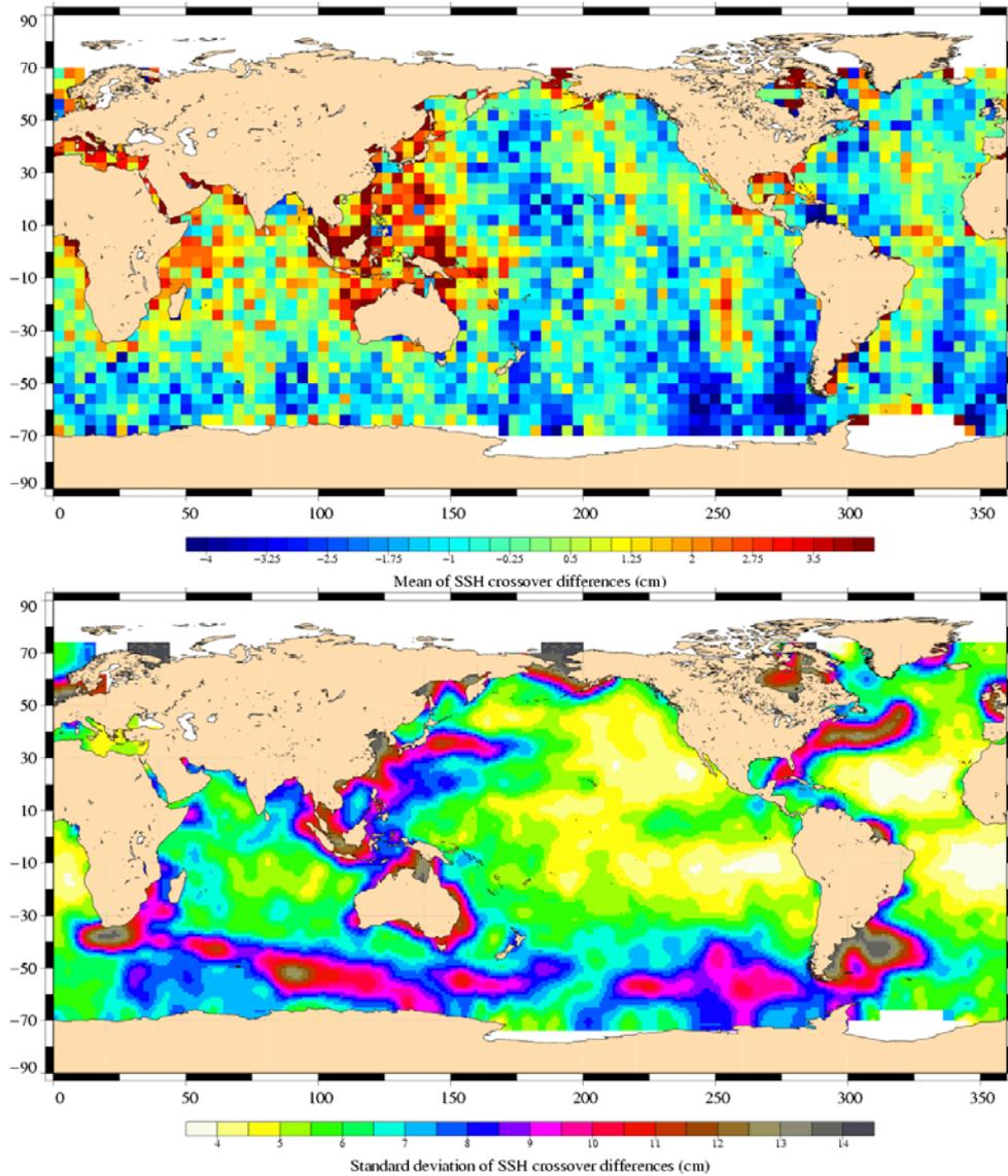
**Figure 87 : Geographical pattern (4x4 degree bins) of crossover [Envisat – Jason-1] mean and standard deviation SSH differences (cm), from cycle 15 to cycle 18**
