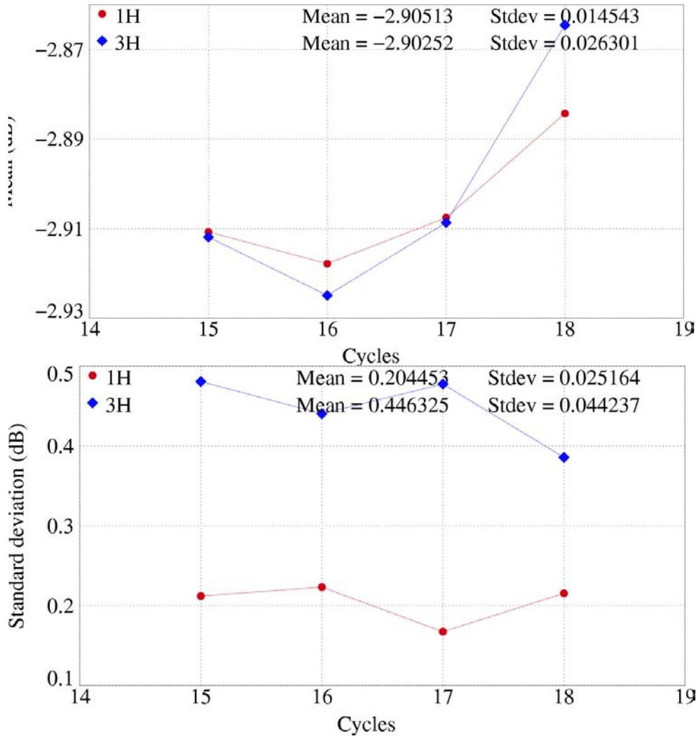
**Figure 82 : Mean and standard deviation of [Envisat – Jason-1] Ku Sigma0 differences at crossover (dB)**
