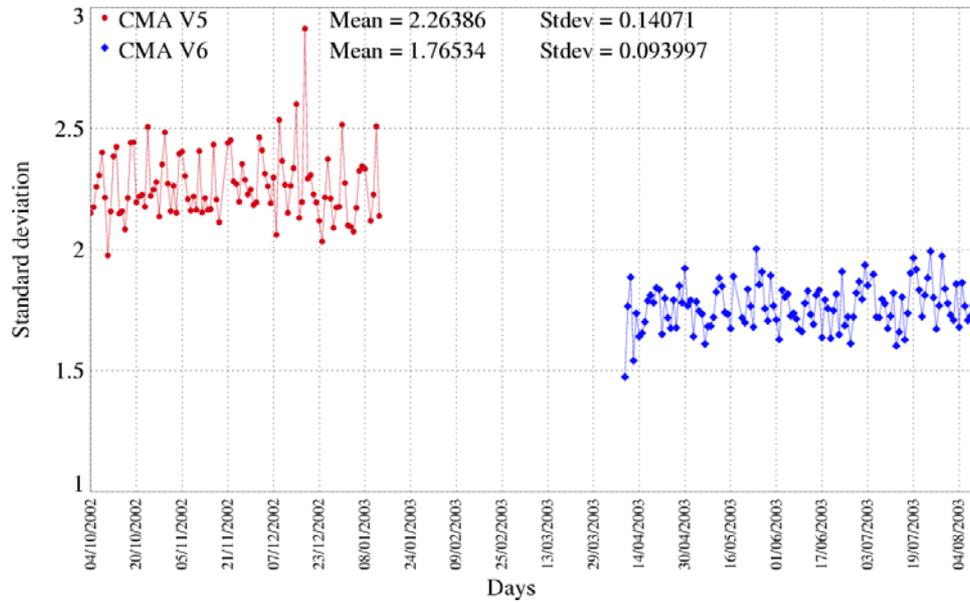
**Figure 25 : Standard deviation of MWR-ECMWF model differences (cm)**
