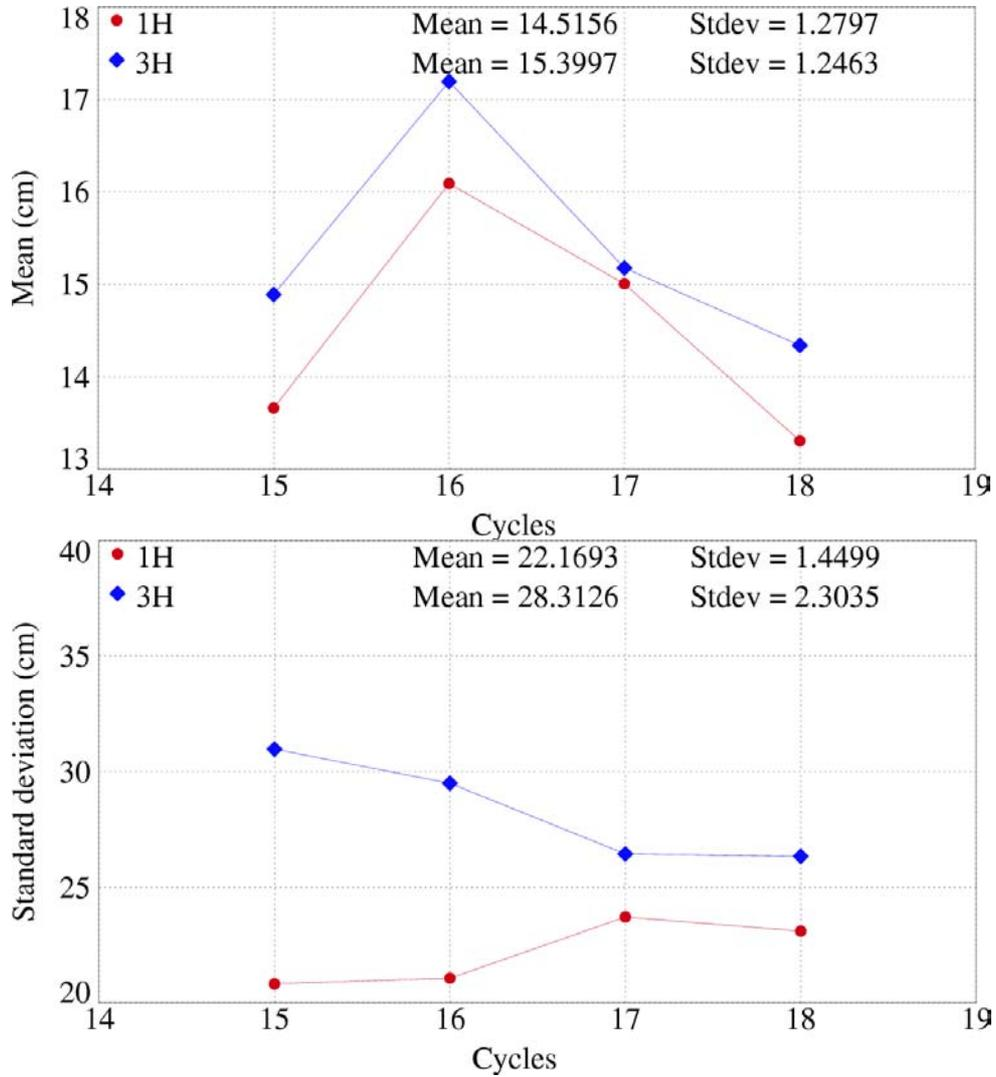
**Figure 81 : Mean and standard deviation of [Envisat – Jason-1] Ku SWH differences at crossover (cm)**
