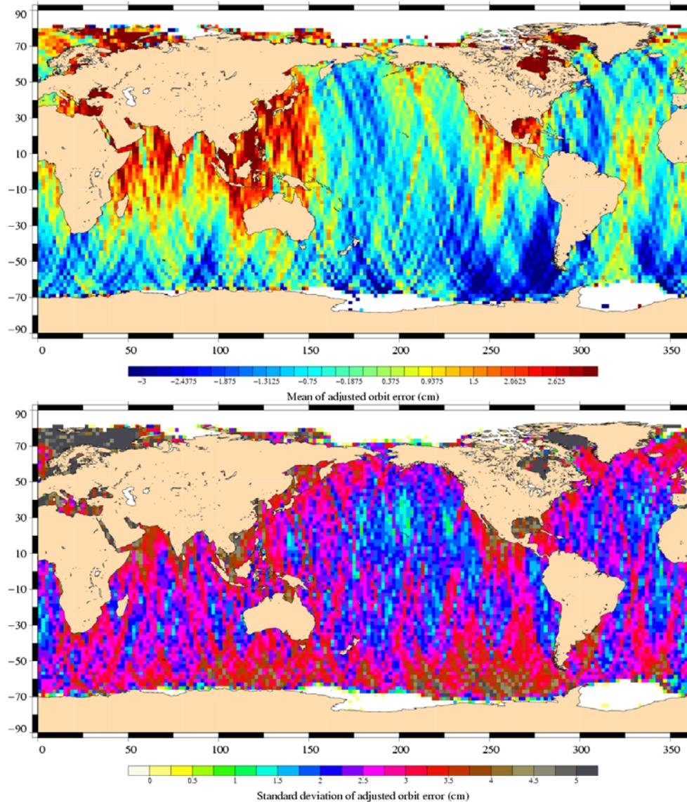
**Figure 88 : Geographical pattern (2x2 degree bins) of mean (centred about the Global mean value) and standard deviation of the Envisat adjusted long wave length error (cm), from cycle 15 to cycle 18**
