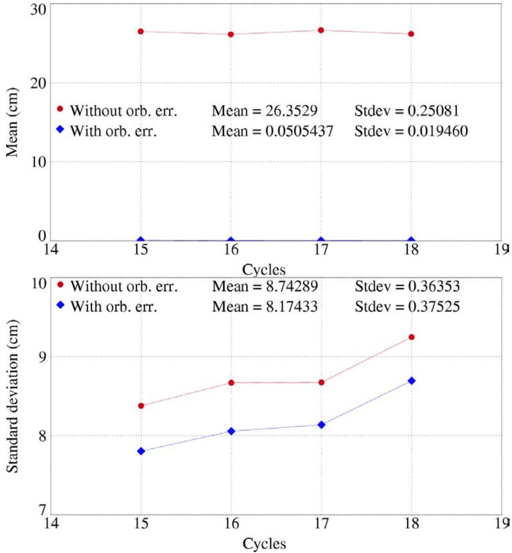
**Figure 89 : Mean and standard deviation of [Envisat – Jason-1] SSH differences at crossover using adjusted long wave length error (cm)**
