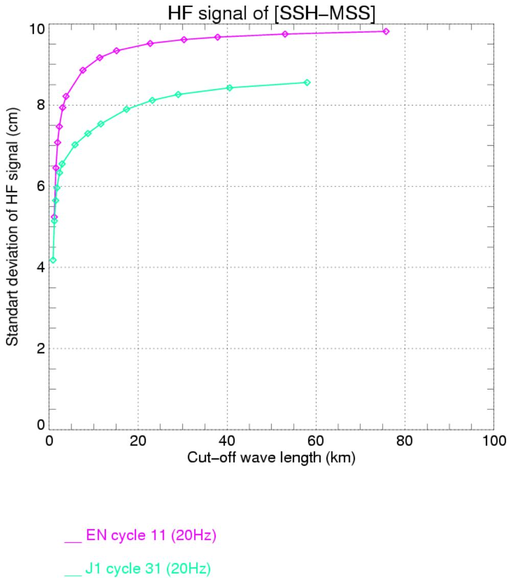
**Figure 58 : Standard deviation of HF[SLA<sub>nc/mss</sub>] at 20Hz according to cut-off wave-length**
