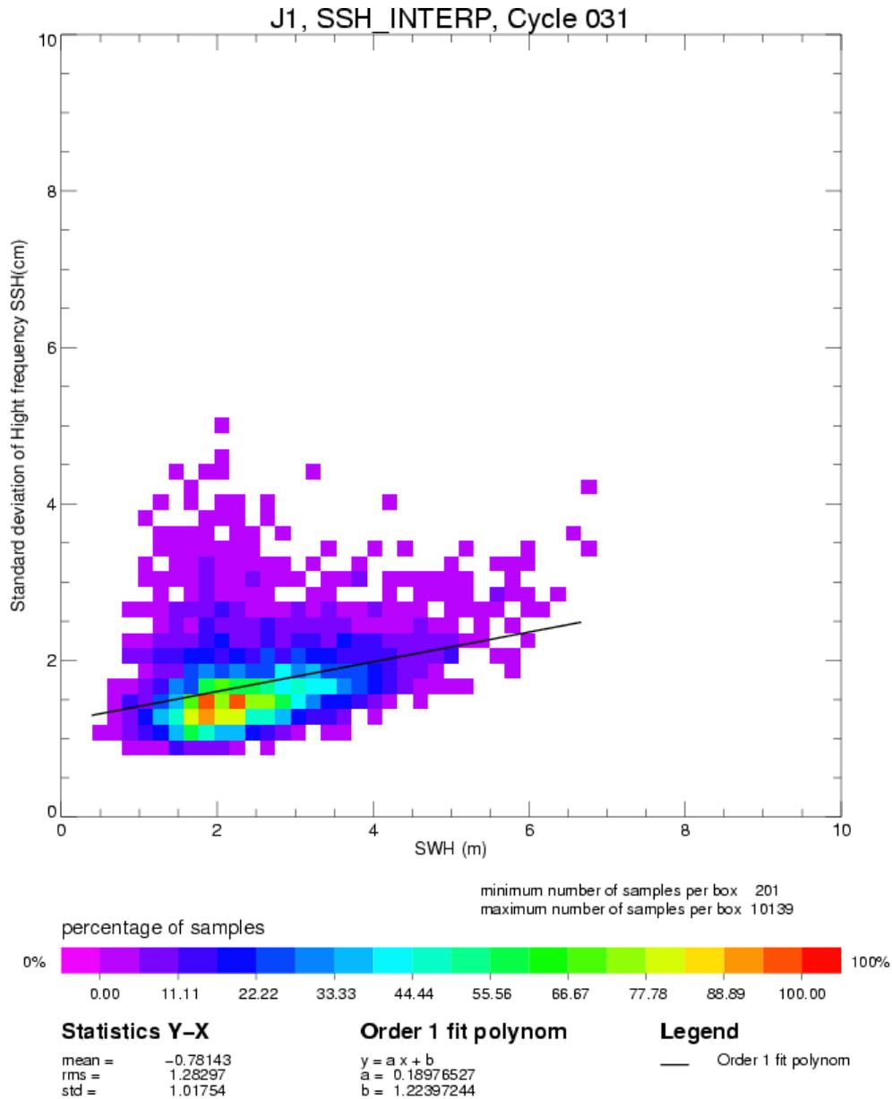
**Figure 75 : Scatter plot of the standard deviation of Jason HF[SLA<sub>nc/mss</sub>] at 1Hz according to waves**
