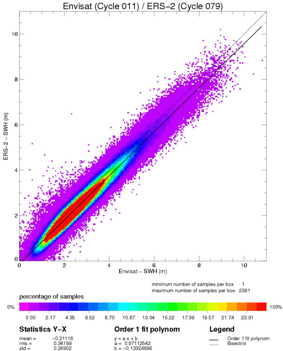
**Figure 94 :** Scatter plot of ERS-2 SWH versus ENVISAT SWH in meters.
