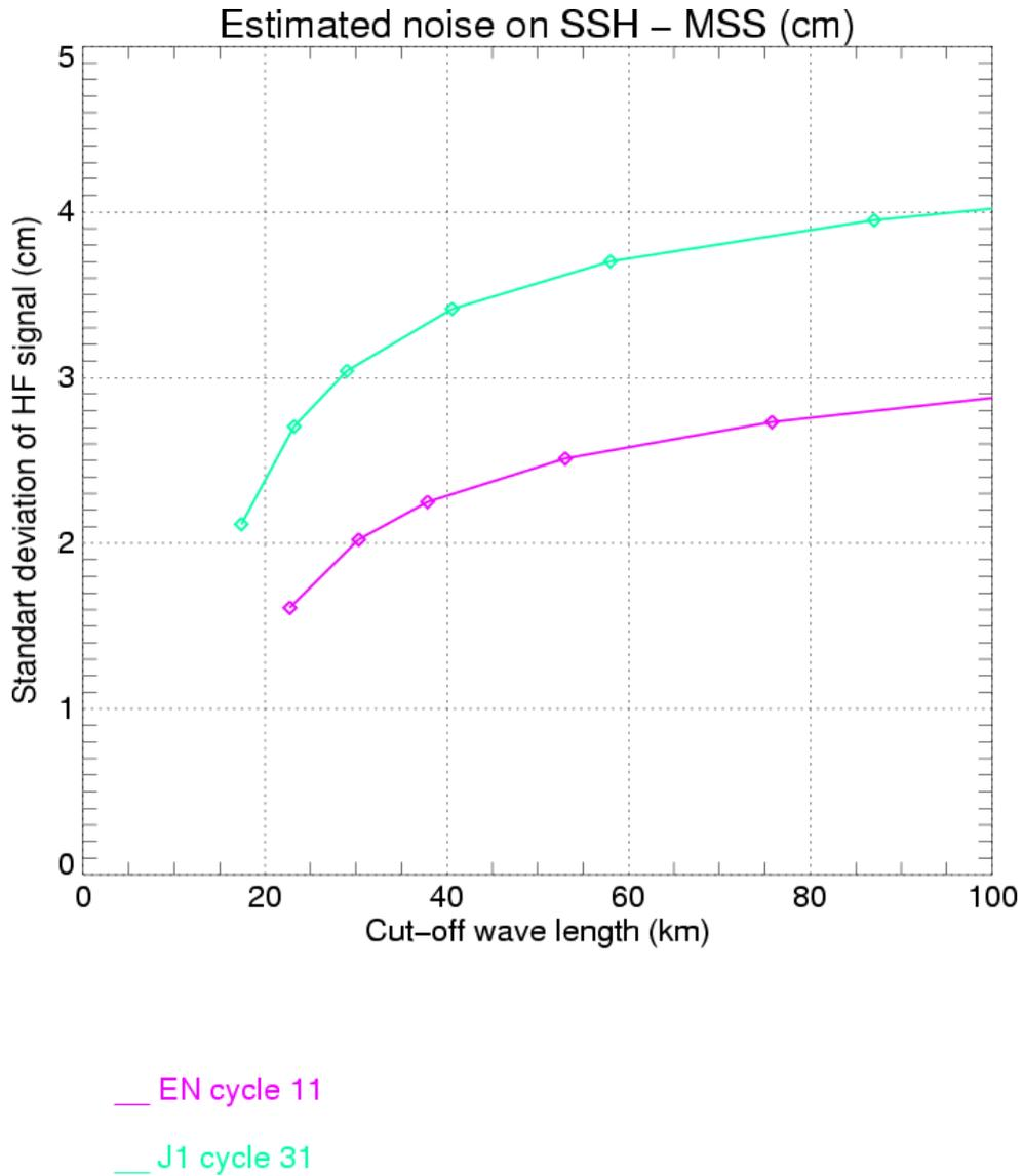
**Figure 67 : Standard deviation of High Frequency signal as a function of the cut-off wave-length, using 1Hz data**
