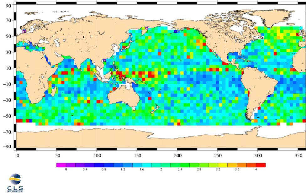
**Figure 72 : Standard deviation of Jason-1 HF[SLA<sub>nc/mss</sub>] at 1Hz**
