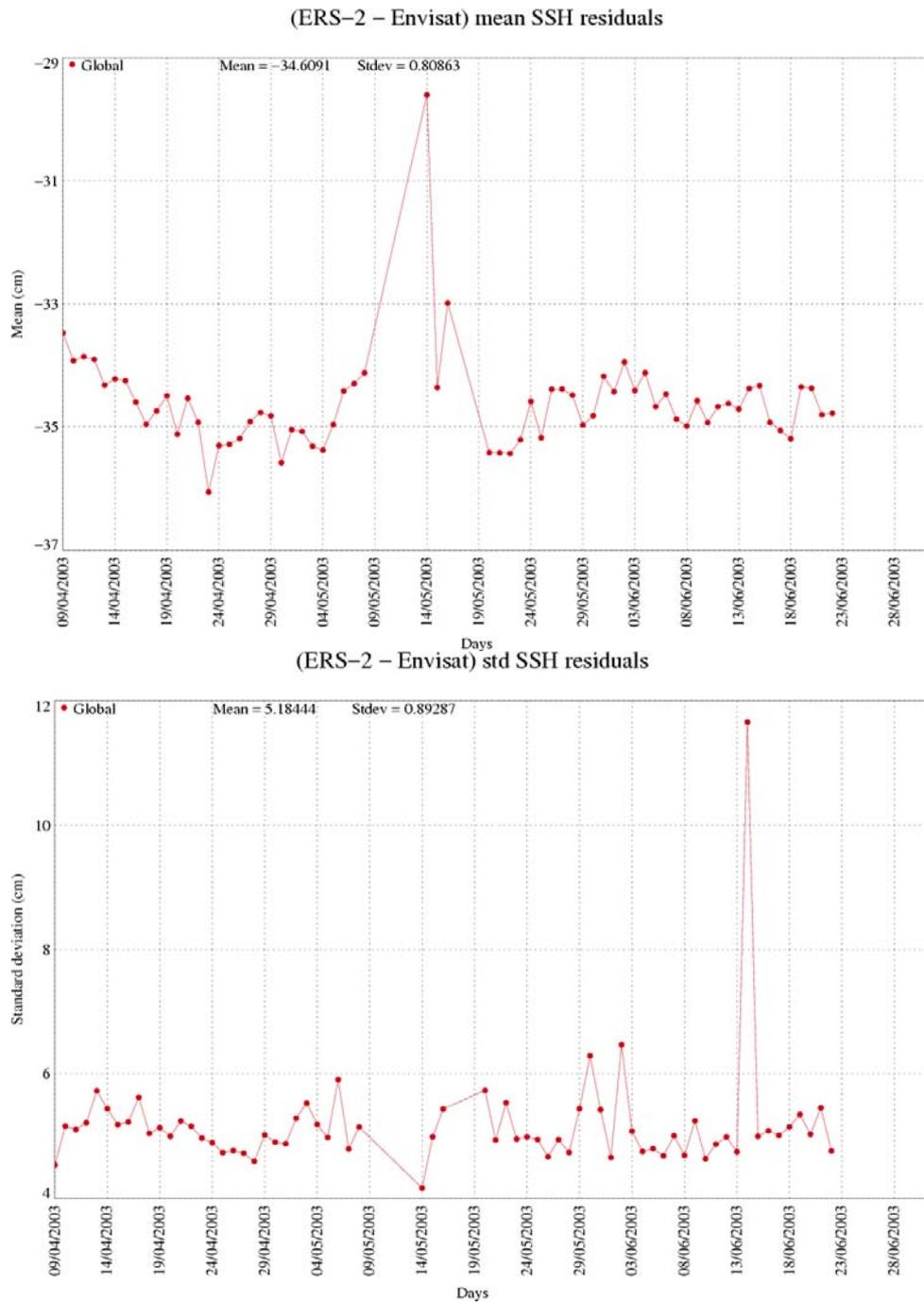
**Figure 103 : Mean and standard deviation of (ERS-2 – Envisat) SSH along track residuals for each day from cycle 15 to 17.**
