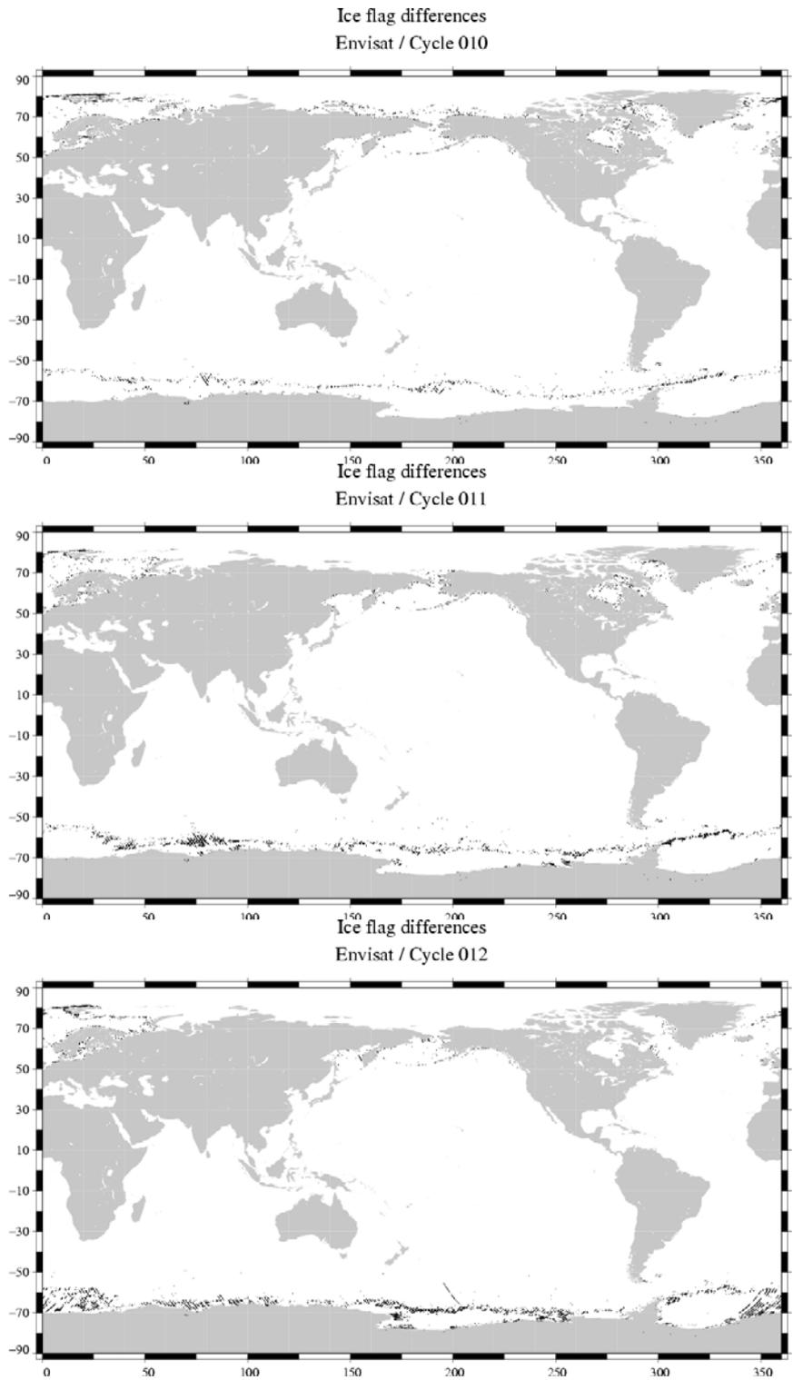
**Figure 55 : Points detected as ice by a 2.0 threshold on peakiness, but seen as ocean data by the ERS-2 method, cycles 10, 11 and 12**
