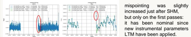
mispointing was slightly increased just after SHM, but only on the first passes: it has been nominal since new instrumental parameters LTM have been applied.
