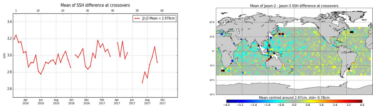
Figure 5 – Cyclic monitoring of Jason-2 - Jason-3 SSH crossover differences mean (left) and map over cycle 1 to 58 (right). Only data with  $|\text{latitude}| < 50^\circ$ , bathymetry  $< -1000\text{m}$  and low oceanic variability were selected.
