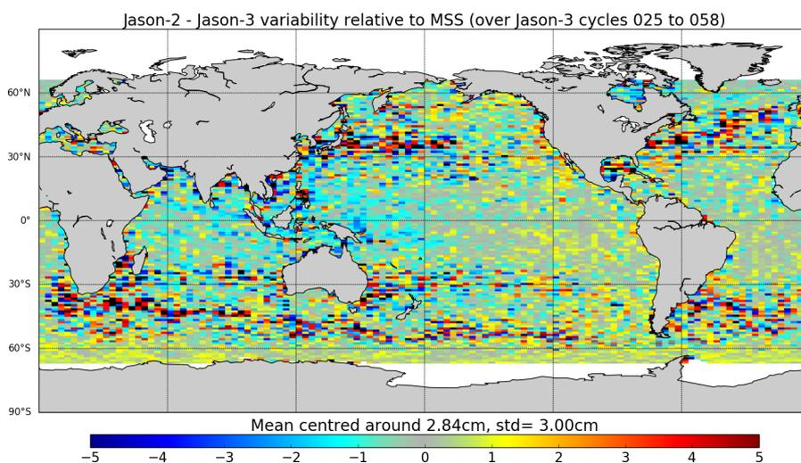
Figure 3 – GDR data. Map of Jason-2 and Jason-3 SLA differences for Jason-3 cycles 025 to 058
