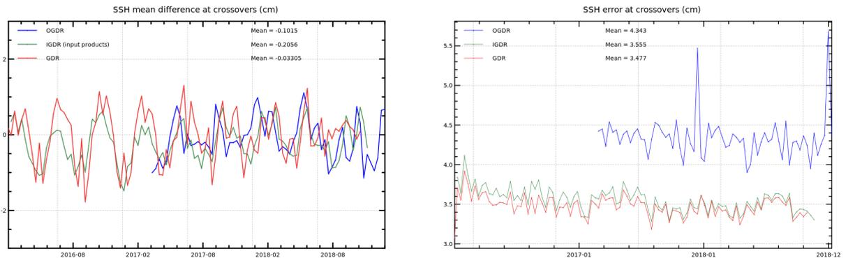
Figure 4 – Monitoring of SSH difference at crossovers for Jason-3 **OGDR**, **IGDR** and **GDR**. Mean of difference (**left**) and error at crossovers (**right**). Only data with  $|\text{latitude}| < 50^\circ$ , bathymetry  $< -1000\text{m}$  and low oceanic variability were selected.
