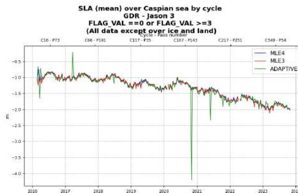
Figure 67 – Cyclic mean of along-track SLA over Caspian sea for MLE3, MLE4 and ADAPTIVE retracking
