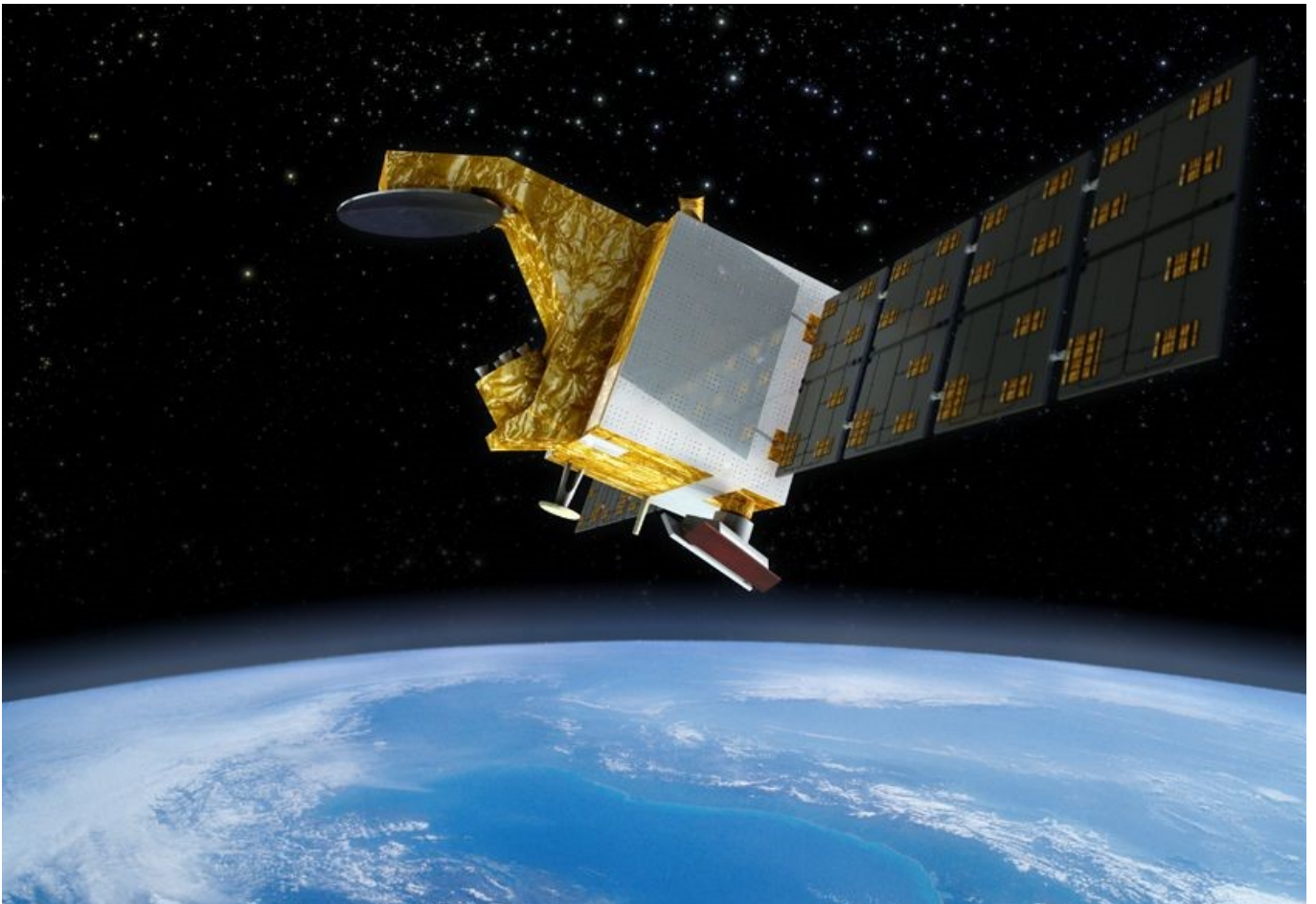
Figure 1. Artist view of the CFOSAT satellite © CNES/Gekko. The SWIM antenna is on the left (six feed horns mounted on a rotating baseplate and illuminating a parabola oriented towards the Earth surface) and the SCAT antenna is at the bottom right (two rectangular slotted waveguide antennas, one for HH and one VV polarization).
