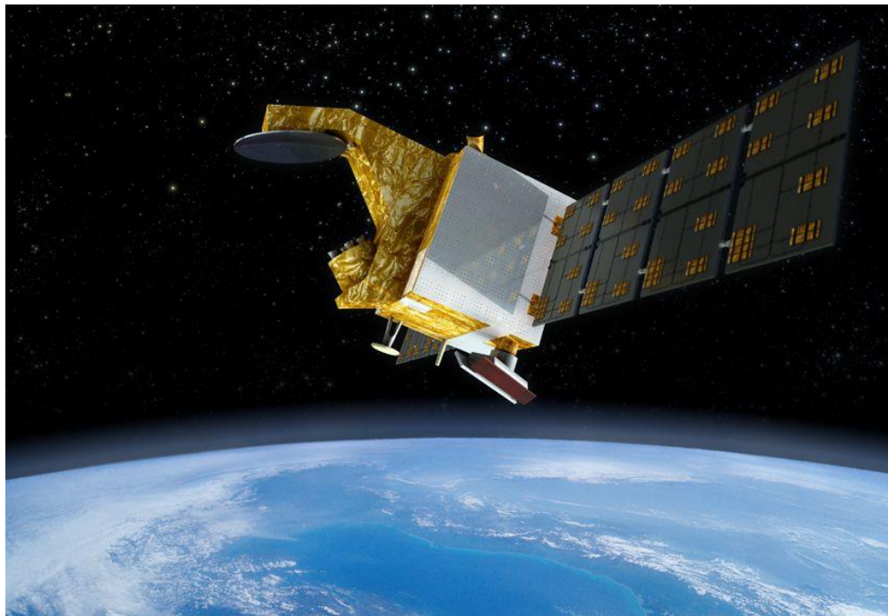
Figure 1. Artist view of the CFOSAT satellite © CNES/Gekko. The SWIM antenna is on the left (six feed horns mounted on a rotating baseplate and illuminating a parabola oriented towards the Earth surface) and the SCAT antenna is at the bottom right (two rectangular slotted waveguide antennas, one for HH and one VV polarization).
