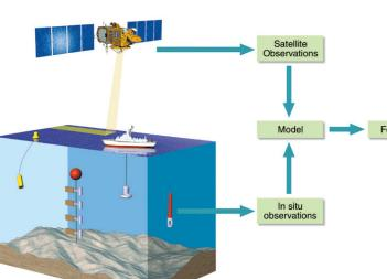
Satellite measurements are complemented by in situ data that enable us to plumb the ocean depths and validate and calibrate satellite instruments. Largescale international programmes such as ARGO are now taking shape to provide the widest possible coverage of the oceans by in situ instruments, to complement spaceborne programmes.
