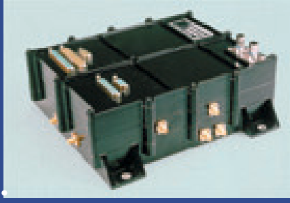
DORIS receiver (Thomson-Detexis) - Flight model.
