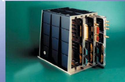
POSEIDON-2 altimeter processing unit (Alcatel) - Flight model.
