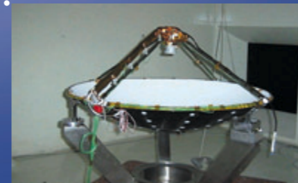
Altimeter antenna (Alcatel) - Flight model in preparation for thermal and mechanical tests.
