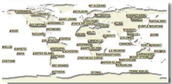
A network of 60 **DORIS ground stations** around the globe provides reference points for continuous tracking of satellite trajectories.
