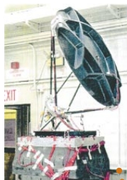
Radiometer (NASA/JPL). Measures atmospheric water vapour.
