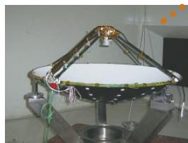
Altimeter antenna (ASPI). Transmits and receives radar altimeter signals at satellite nadir.
