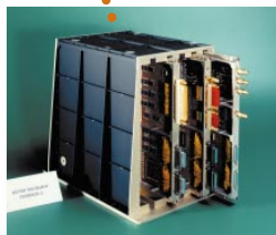
POSEIDON 2 altimeter processing unit (ASPI). Measures satellite-to-ocean range.
