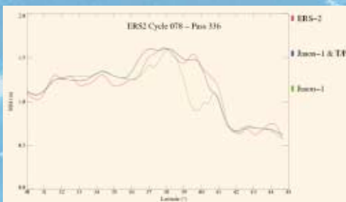
Comparison with the sea level observed along an ERS-2 track (black track in maps, right). The Jason-1 and Topex/Poseidon tandem mission is able to reproduce most of the signals observed by ERS-2, while the Jason-1 data alone missed several important Gulf Stream meanders (e.g. 39-40°N, with sea level height of about 40 cm).
