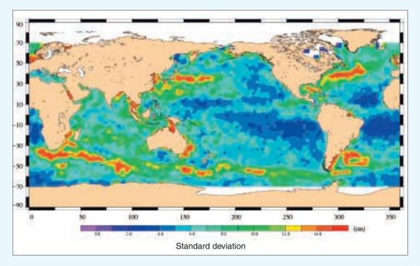
Figure 2. RMS of sea level anomalies computed from 21 cycles of Jason-I IGDR data (units are cm)
