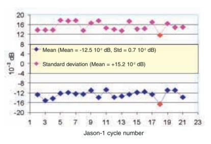
Figure 1. Mean and RMS of sigma0 differences between Topex/Poseidon and Jason-1 (Units are dB) (On the "Mean" curve, blue diamonds are Topex measurements, while the red one refers to Poseidon-1 )
