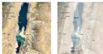
Classical altimetry vs Swot around the Dead Sea (left, classical altimetry, measurements are only under the colored lines ; right, with Swot, measurements are all over the whitened areas)
